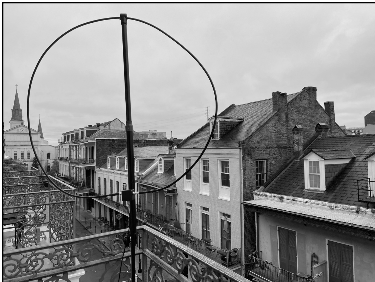
Figure 1: The author's W6LVP loop perched on a balcony overlooking the French Quarter in New Orleans, Louisiana.
