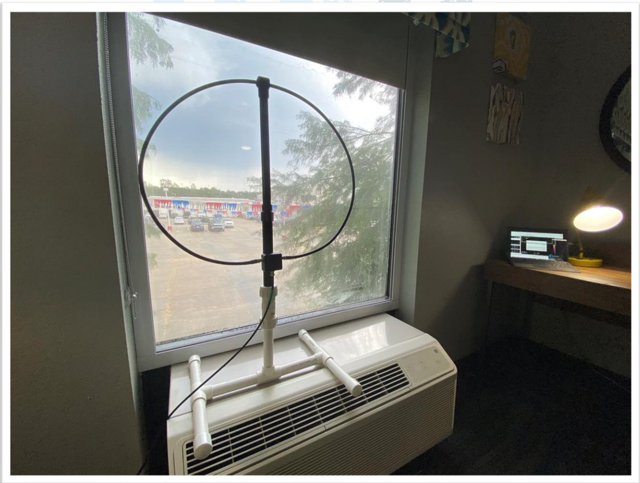
1: The portable W6LVP loop antenna and PVC stand as deployed in a hotel room, similar to the setup used in Lake Forest. The Surface Pro running SDR Console is seen on the desk.
